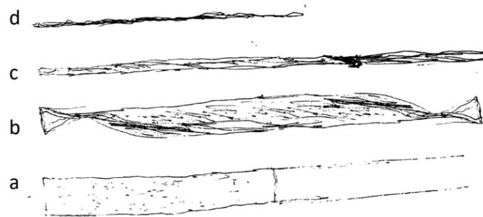
Closing conditions of the ends tests whether the twisted strips would uncurl. Tied ends creates a bulkier but more reliable condition. Rolled strips (e) in one direction has a less reliability in keeping the strip in place as opposed to opposite twisting (b, c, d).
