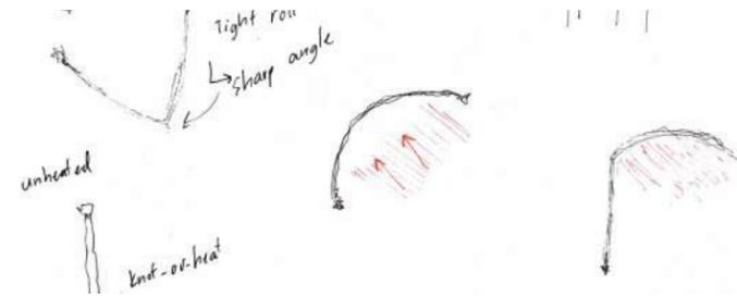
Tests of shrink wrap involve preheating before twisting and post-heating. Plastic strips curl towards heat source
