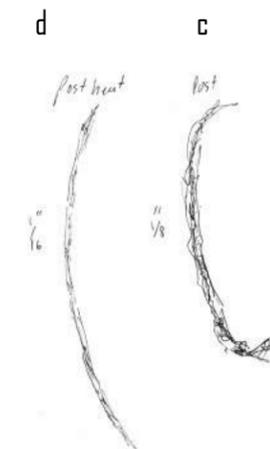
Sequence and order affect the quality of the shrink wrap. The wrinkles caused by early heating creates a thicker condition than the preheated state.
